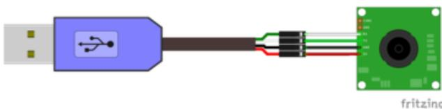
**Camera Vin to USB 5V or 3V** (red wire on USB console cable)
