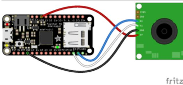
**Camera 5V to board USB or 5V power** (note this means you must have the board plugged into a USB / 5V power supply to properly power the camera).
