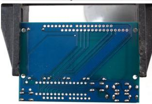
Solder each leg, taking care not to accidentally 'short' two button legs together. The ones for the directional pads are very close!
