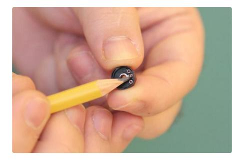
This... is a better way to fly. The foil contact and limiter are pressed into place - give them a little wiggle towards the gears and they should come right off.
