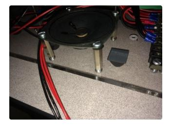
Prepare the speakers for mounting by attaching 4 M4 standoffs with M4 screws to the bottom of each speaker like so. I added rubber washers between the speaker and the standoffs, hoping that this would prevent any strange vibrations. I'm not sure if it does the least bit of good.
