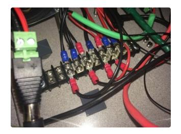
A picture is a thousand words. Here you can see the barrier block, the jumper blocks (the metal tabs that stick up and over, as well are the crimp connectors used to attach the wires to the barrier block.
