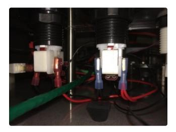
The illumination is easy. To save on using any 'active' components, these are just wired straight to the power bus.
