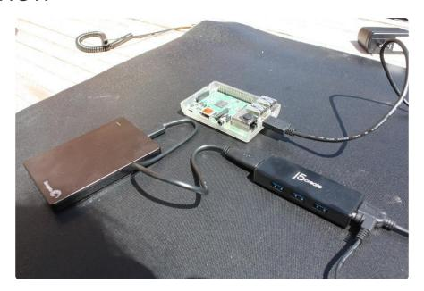
One of the more noticeable limitations of the Raspberry Pi is using an SD card for its main storage. If you've been using a Pi for a while, you might be looking for more storage, faster access times, or media with a longer lifespan than many SD cards turn out to have.
