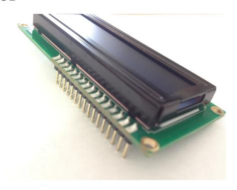
Whenever you come across a LCD that looks like it has 16 connectors it is most likely using a HD44780 controller. These devices provide the same pinouts making them relatively easy to work with. The LCD uses a parallel interface meaning that we will need many pins from our raspberry pi to control it. In this tutorial we will use 4 data pins (4-bit mode) and two control pins.
