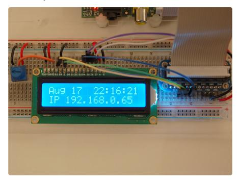
The following code can be downloaded to your raspberry pi and run to get the date, time and IP address of your machine on the LCD display.
