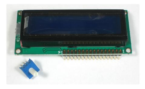
Next you'll need to solder the header to the LCD. You must do this, it is not OK to just try to "press fit" the LCD!
