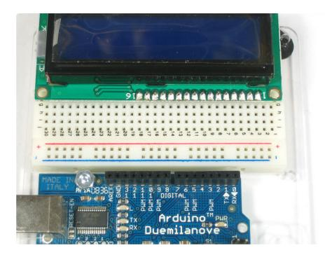
Start by connecting the **5V** and **GND** wires from the cobbler to the breadboard. Then connect pins #1, #2 and #15, #16 to the breadboard power rails as shown. The backlight should come on. If it doesn't, check the wiring!
