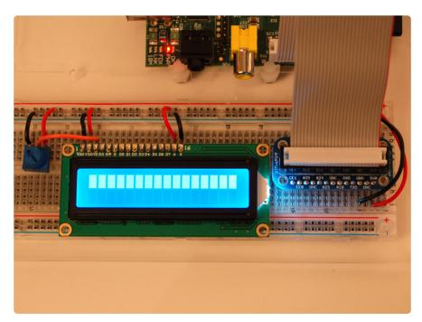
Finish the wiring for the RS, RW, EN, D4, D5, D6, and D7 pins as shown in the diagram up top.
