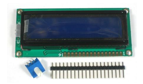
Most LCDs have a strip of 16 pins on the top, if the header is a little longer, just break it off until its the right length
