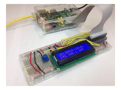
Adding a LCD to any project immediately kicks it up a notch. This tutorial explains how to connect an inexpensive HDD44780 compatible LCD to the Raspberry Pi using 6 GPIO pins. While there are other ways to connect using I2C or the UART, this is the most direct method that gets right down to the bare metal.
