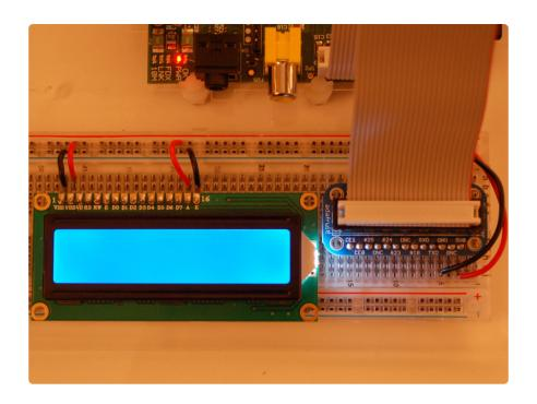
Next, wire up the contrast potentiometer as shown above, with the middle pin connecting to LCD pin #3 and the other two pins going to 5V and ground.
