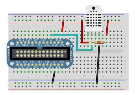
Time to start exploring more sensors with the Raspberry Pi and Beaglebone Black! Today we'll be checking out the <u>DHT11</u> (http://adafru.it/386), <u>DHT22</u> (http://adafru.it/385) and <u>AM2302</u> (http://adafru.it/393) humidity and temperature sensors available from Adafruit
