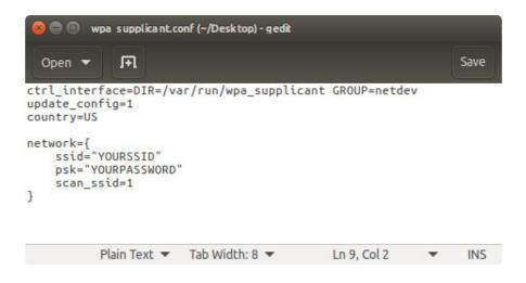
Save the file and safely remove the SD card from your PC. Put it in the Raspberry Pi and power it up. If all goes well, it should copy the file over and connect to your Wifi.
