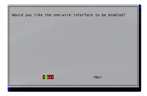
Exit out of raspi-config and reboot your Pi so the 1-wire kernel modules load up.
