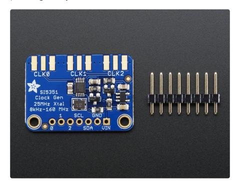
The Si5351 clock generator is an I2C controller clock generator. It uses the onboard precision clock to drive multiple PLL's and clock dividers using I2C instructions. By setting up the PLL and dividers you can create precise and arbitrary frequencies.
