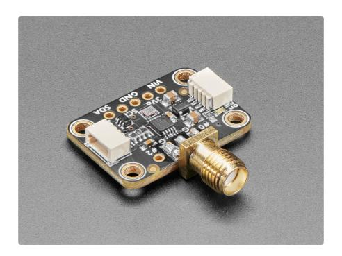
There is a 3.3V LDO regulator so it can be powered from 3-5VDC. We also put level shifting circuitry on the I2C lines so you can use this chip safely with 3V or 5V logic.
