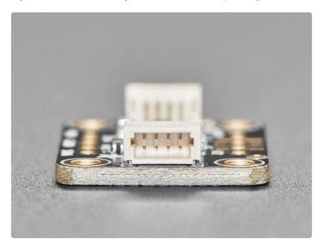
On the PCB in the <u>STEMMA QT form factor</u> (https://adafru.it/LBQ), there are <u>STEMMA QT connectors</u> (https://adafru.it/JqB) on either side that are compatible with the <u>SparkFun Qwiic</u> (https://adafru.it/Fpw) I2C connectors. This allows you to make solderless connections between your development board and the Si5351 or to chain it with a wide range of other sensors and accessories using a <u>compatible</u> <u>cable</u> (https://adafru.it/JnB).
