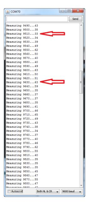
The larger the number the higher the transmission power. For example, 96.3MHz is a higher number than the others (FYI, its Univision 96.3 FM (https://adafru.it/dBs)!) whereas 95.1 MHz is nice as low, that's not used for any transmission. Try to find a number that's also not surrounded by high numbers, since it can get 'drowned out' by the nearby frequencies.
