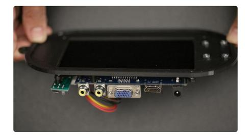
The  $\#2-56 \times 3/8$  screws should thread down into the vr-mnt.stl but not all the way through the part. Insure the screws are tight and all of the components are jiggle free!
