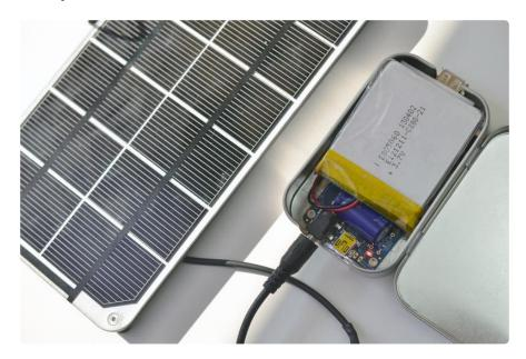
Test your circuit by plugging in the solar panel, then placing it in direct sunlight. The red charging light should be bright and solid, not flashing. To learn more about the charger, check out the <u>LiPoly Charger Guide</u> (). you can also charge your battery using the mini USB jack.
