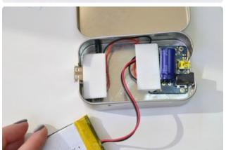
Use the double sided foam tape that came with the MintyBoost kit to secure it to the inside of the mint tin.
