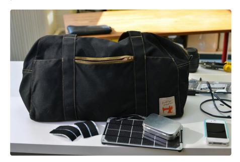
Use two pieces of adhesive Velcro tape to secure the solar panel to your bag. Stick the fuzzy side to your bag neatly and aligned with the size of your solar panel, then mate the scratchy hook side of the Velcro to the fuzzy side, peel off the adhesive back and gently press on your solar panel. Then squish the glue joints before carefully separating the newly affixed Velcro pieces. If necessary, stitch or staple the fuzzy side of the Velcro to your bag.
