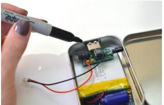
Line the bottom of the mint tin with tape to insulate it from the metal contacts on your circuit board. Also wrap the battery in tape.
