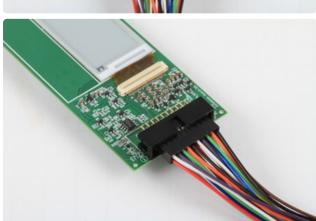
Be sure to center the connector in the socket. The socket is wider than the connector and the display will not work if you plug it in off-center.
