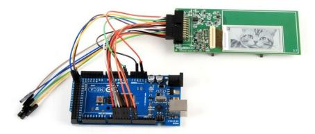
Wiring for the Mega is similar to the Uno and Leonardo. Only the SPI pins are in a different location.
