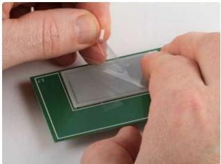
Remove the protective film Lift the white tab and gently peel back the protective film from the display.
