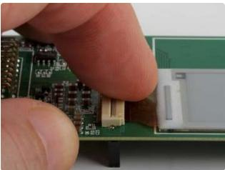
Close the Socket Gently push the socket closed to lock the flex connector in place.
