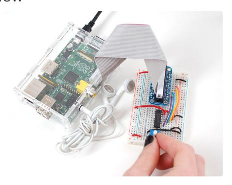
Teaching the Raspberry Pi how to read analog inputs is easier than you think! The Pi does not include a hardware <u>analog-to-digital converter</u> (https://adafru.it/eYp), but an external ADC (such as the <u>MCP3008</u> (http://adafru.it/856)) can be used, along with some SPI code in Python to read external analog devices.
