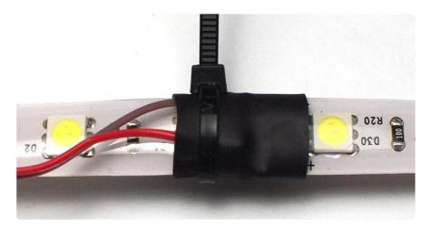
Add a ziptie, some epoxy, or both to provide strain relief and added waterproofing at this delicate spot.
