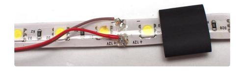
Grab the jack side of the waterproof power connector and solder the red wire to the positive (+) pad on the LED strip, and the black wire to the negative (-) pad. Slide a large piece of heatshrink tubing over the LED strip and the newly formed junctions.
