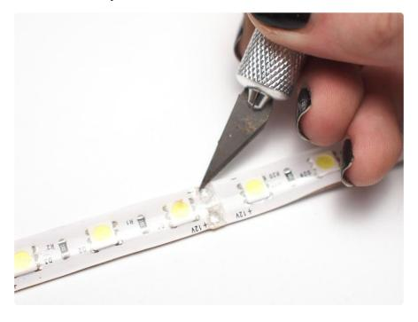
Scrape away the plastic coating over two solder pads at the center of your LED strip.
