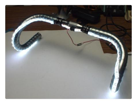
Test out the LEDs with a reliable 12V power source. These drop bars were adorned with 1m of LED strip, while the bullhorns below have 2m spiraled around them.
