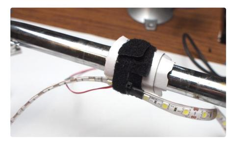
Secure the center of the LED tape to the center of your handlebars, positioned around your stem. If your handlebars aren't attached to a stem when you do this project, add something to occupy its place, like rolled up cardboard and a velcro tie.
