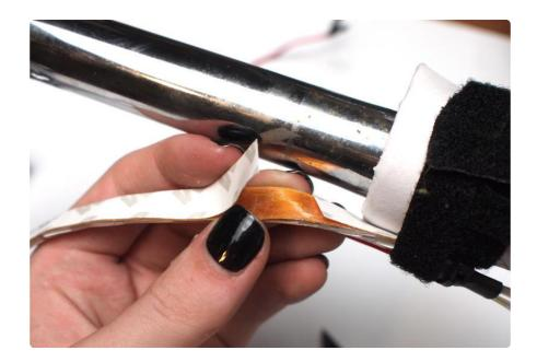
Cut the backing strip near the stem to expose the LED strip's adhesive. Peel away the backing as you affix the strip in position on the handlebars.
