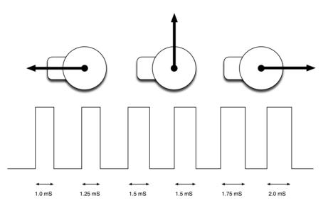
"Continuous" Servos, also called "360 Servos" work very similarly, so you can use them just like a position servo. Instead of the absolute position, a continuous servo will adjust its speed with different pulse widths
