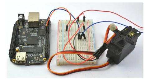
A Python test program will allow you to set the angle of the servo between 0 and 180 degrees.
