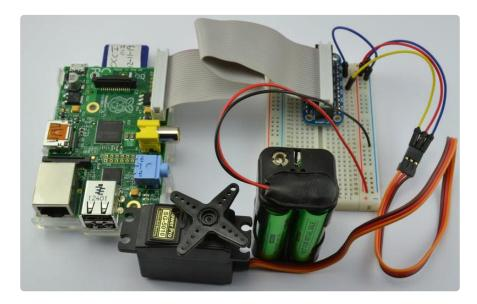
Servo motors are controlled by pulses of varying lengths. This requires fairly accurate timing. The Raspberry Pi has one pin that generates pulses in hardware, without having to rely on the operating system.
