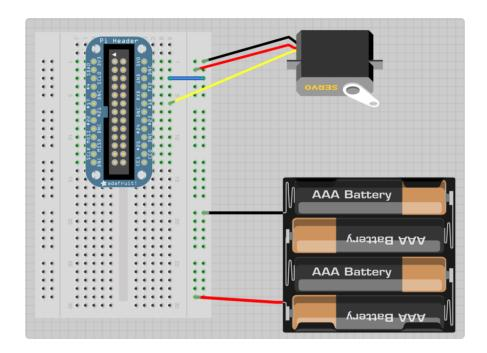
The Pi Cobbler is used to link the Raspberry Pi to the breadboard. If you have not used the Cobbler before take a look at Lesson 4 () in this series.
