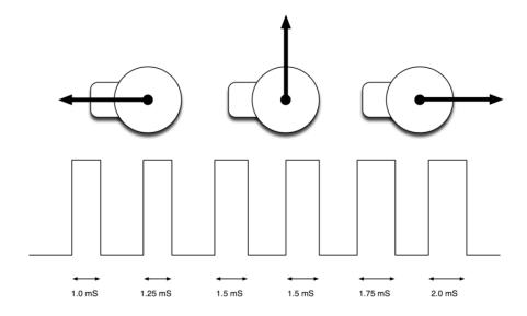
The end points of the servo can vary and many servos only turn through about 170 degrees. You can also buy 'continuous' servos that can rotate through the full 360 degrees.
