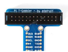
Start by putting the PCB in front of you with the text as shown on the left. Then place the header on top.
