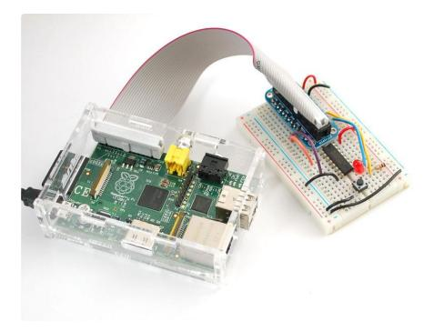
Now that you've finally got your hands on a Raspberry Pi® (), you're probably itching to make some fun embedded computer projects with it. What you need is an add on prototyping Pi Cobbler from Adafruit, which can break out all those tasty power, GPIO, I2C and SPI pins from the 26 pin header onto a solderless breadboard. This mini kit will make "cobbling together" prototypes with the Pi super easy.
