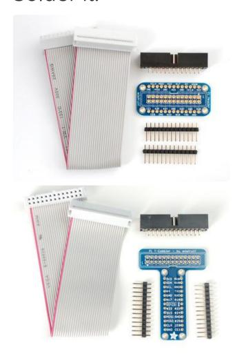
First up, open up your kit and verify you have the components - gray cable, blue PCB, black connector and a stick of male header. The header is breakaway, so it might be one long piece instead of two shorter
