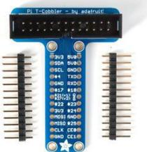
Next break the long piece of header into two 13 pin pieces. You can do this with diagonal cutters, pliers or your fingers
