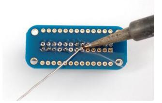
With your soldering iron heated up to 700 degrees F, and some solder, heat up each ring/pin pair for 2 seconds, then poke the end of the solder in to melt it in and make a strong electrical and mechanical connection. Then pull the solder away. Finally remove the iron.
