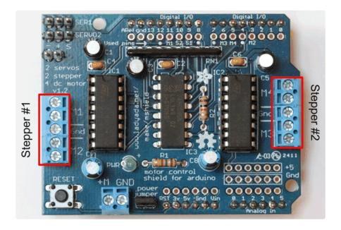
AF\_Stepper Stepper1(48, 1); // A 48-step-per-revolution motor on channels 1 & amp; 2 AF\_Stepper Stepper2(200, 2); // A 200-step-per-revolution motor on channels 3 & amp; 4
