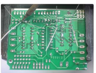
Next are the three 100uF electrolytic capacitors C1, C3and C5. Electrolytic capacitors are polarized and must be placed in the correct orientation or they could pop! The long leg of the capacitor is the positive (+) leg and goes into the hole marked with a +. The close-up images shown here indicate with hole is the + one.
