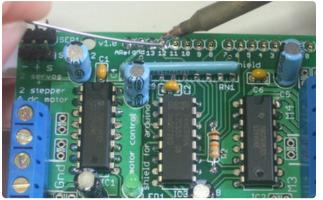
Solder in each pin of the header.
