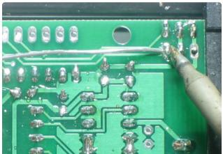
Solder in the 3 pieces of header and the three terminal blocks.
