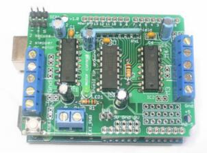
Next, place the 8-pin and 6-pin headers into the Arduino board. This will make sure that the headers are perfectly lined up.
